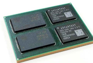
A test processor designed for V93000 EXA Scale test system developed jointly by Germany and Japan
