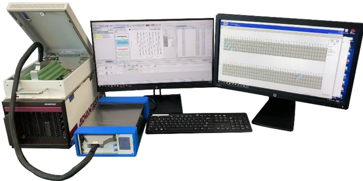
LXI Modular Chassis, Switch modules and EVA100 Measurement System
