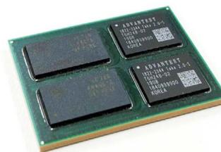
A test processor designed for V93000 EXA Scale test system developed jointly by Germany and Japan
