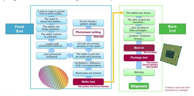
In semiconductor testing, electrical signals are applied to semiconductor devices, and the output signals are compared with reference data and expected values to determine whether the device has passed or failed. Semiconductor manufacturing is said to involve more than 1,000 individual process steps. Among these steps, semiconductor testing is the only process that uses electrical signals to test devices, playing a critical role in quality assurance.
