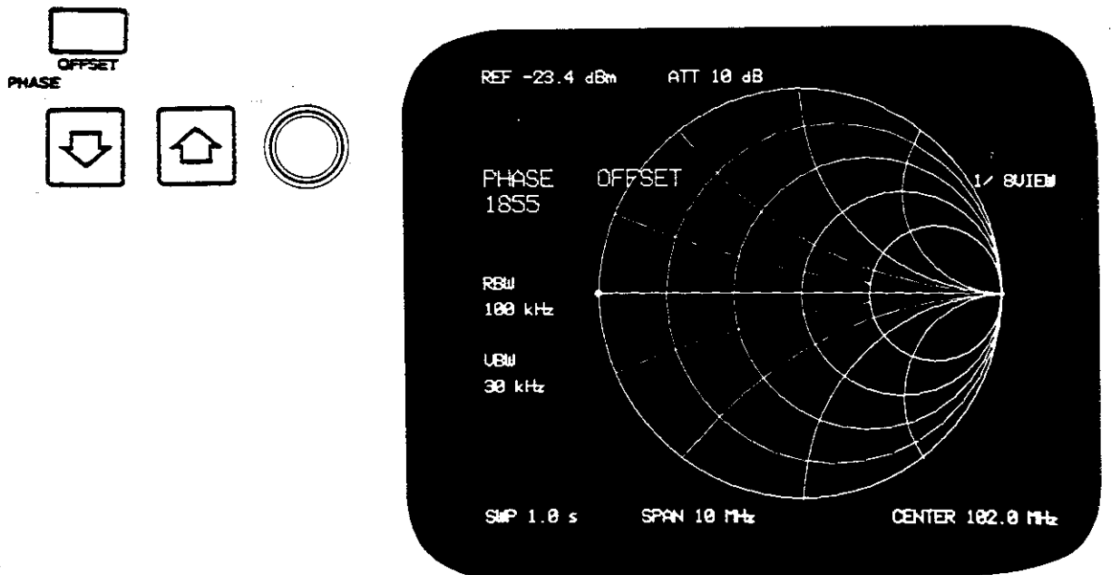
Fig. 9-10 Calibration for DUT terminal shorted
