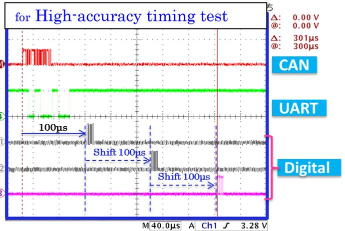
Figure 3. High accuracy timing signal
