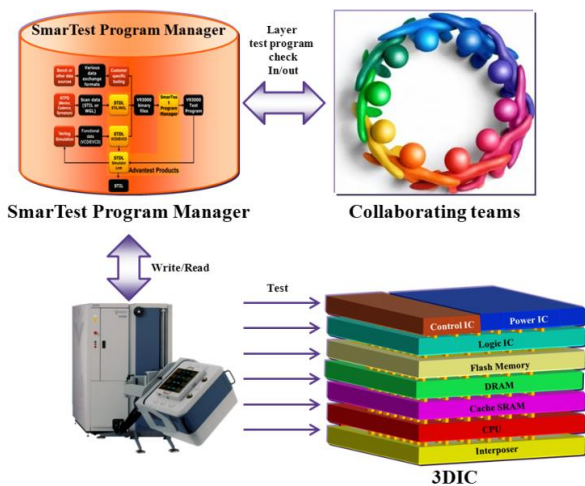
Figure 2 SmarTest Program Manager facilitates collaborative program development.
