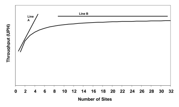
**Figure 3** Throughput as a function of number of sites in the test cell showing the two regions of behavior; A. linearly-increasing throughput with increased number of sites and B. asymptotic region at which little or no gain in throughput is realized.
