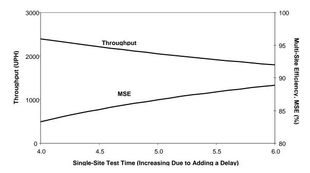
**Figure 1** Graphical representation of data from Table 2, showing increasing of multi-site efficiency at the expense of decreased throughput.
