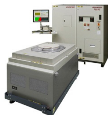
T5833 for DRAM and NAND Flash Memory DRAM・NANDフラッシュ向け
