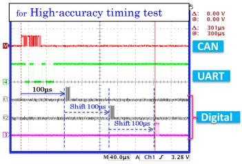
Figure 3. High accuracy timing signal
