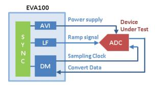
**AVI:** Voltage current monitor/source module **LF:** AWG, 24-bit resolution, THD -100 dB typ **DM:** Digital module, histogram calculation
