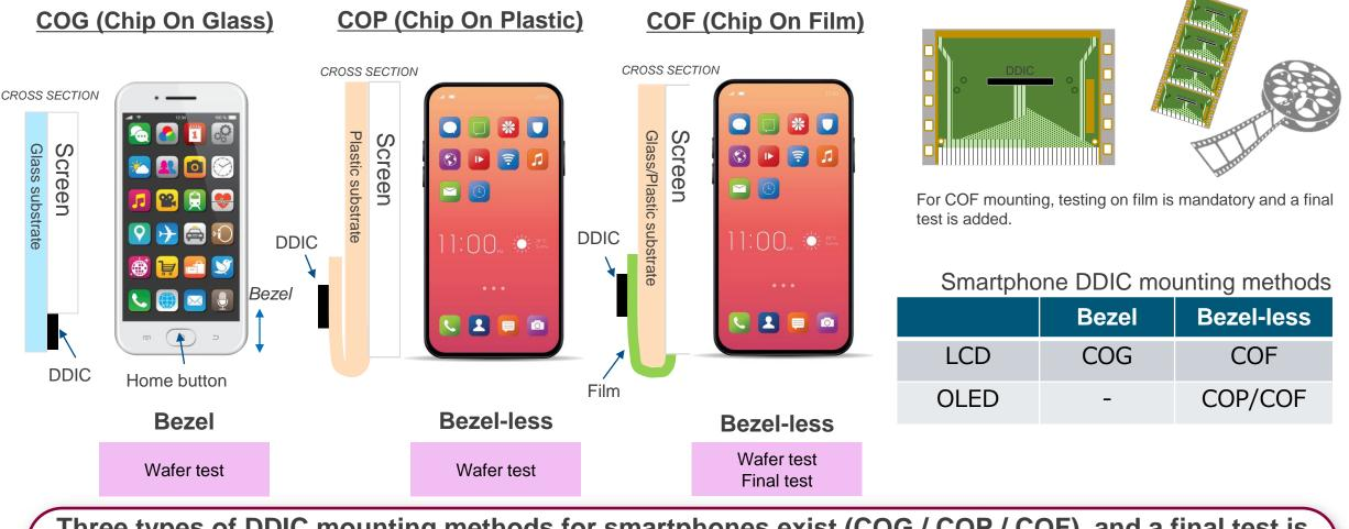
Three types of DDIC mounting methods for smartphones exist (COG / COP / COF), and a final test is added for COF
